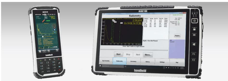
Detection device in a shock-resistant, dust-and-moisture-proof container registers gamma radiation of controlled radionuclides.
