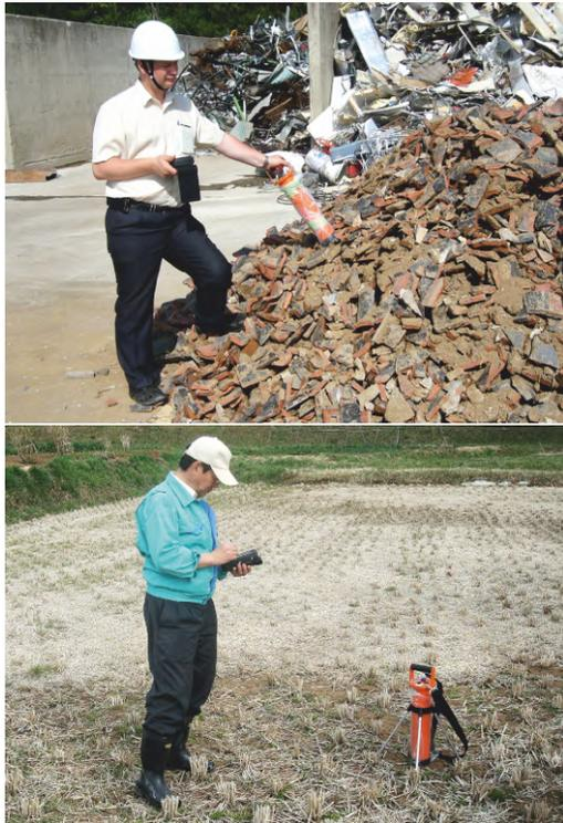
**Radiation background measurement and no-sampling radiometry**
