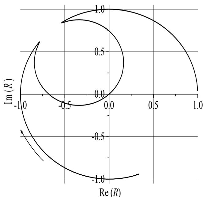
*Fig. 1. The behavior of real and imaginary parts of the resonance reflection amplitude  $R$  near the resonance depending on the molecule energy. The arrow indicates the direction of the moving with the energy increase.*
