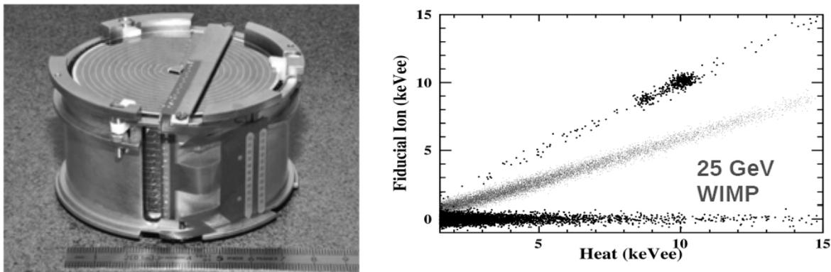
Fig. 1. Left: Photo of FID800 detector. Right: Ionization and heat for events registered with EDELWEISS-III (30 kg.d) – black dots, and expected event band (MC) for light WIMPs (for  $M_{\text{WIMP}} 25 \text{ GeV}/c^2$ ) – tiny gray dots.
