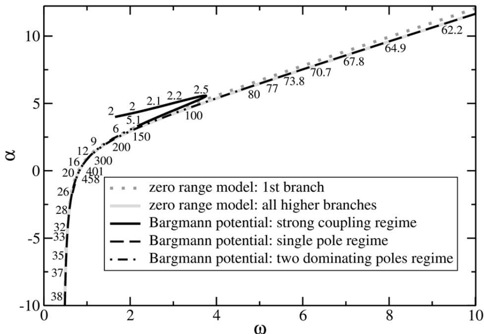
*Fig. 1. The modified Phillips line: the universal correlation between the low-energy properties of three-body systems. The numbers along the curve mark the corresponding value of the two-body scattering length.*
