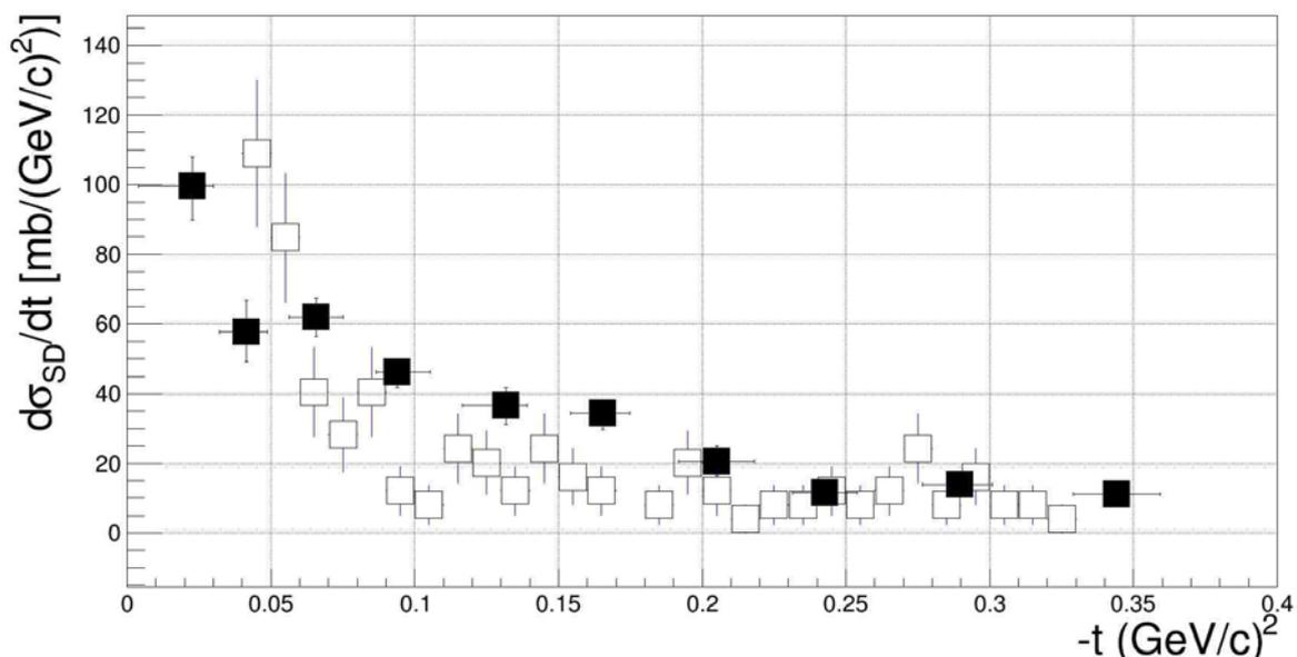
Fig. 1. Differential diffraction cross-section of the reaction  $pA \rightarrow pX$  for the nuclear target Al.
