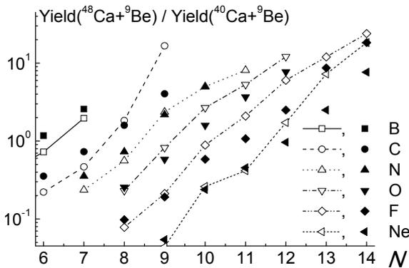
Fig. 1. Yield ratios for different elements for the reactions  $^{48}\text{Ca}$  and  $^{40}\text{Ca}$  on  $^9\text{Be}$  at 140 MeV / nucleon. The closed symbols are the experimental results, while the curves with open symbols are the calculations.
