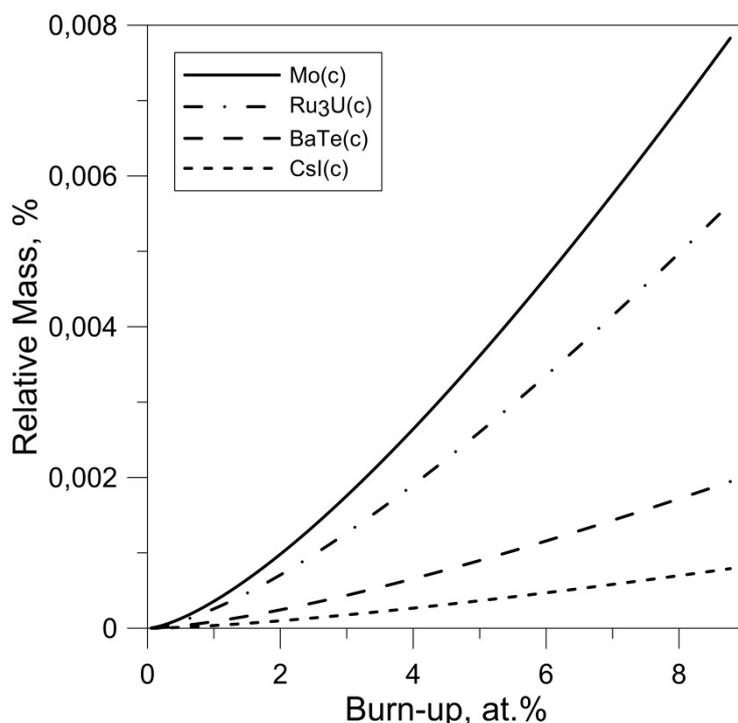
Fig. 1. Evolution of Mo(c) and Ru<sub>3</sub>U(c) phase during irradiation of UN fuel at T = 1200 K.
