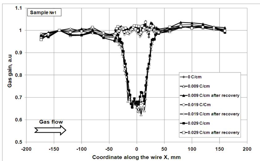
Fig. 1. Gas gain distribution along the straw measured on aged and then on recovered straw in 60%Ar + 30%CO<sub>2</sub> + 10%CF<sub>4</sub> gas mixture.
