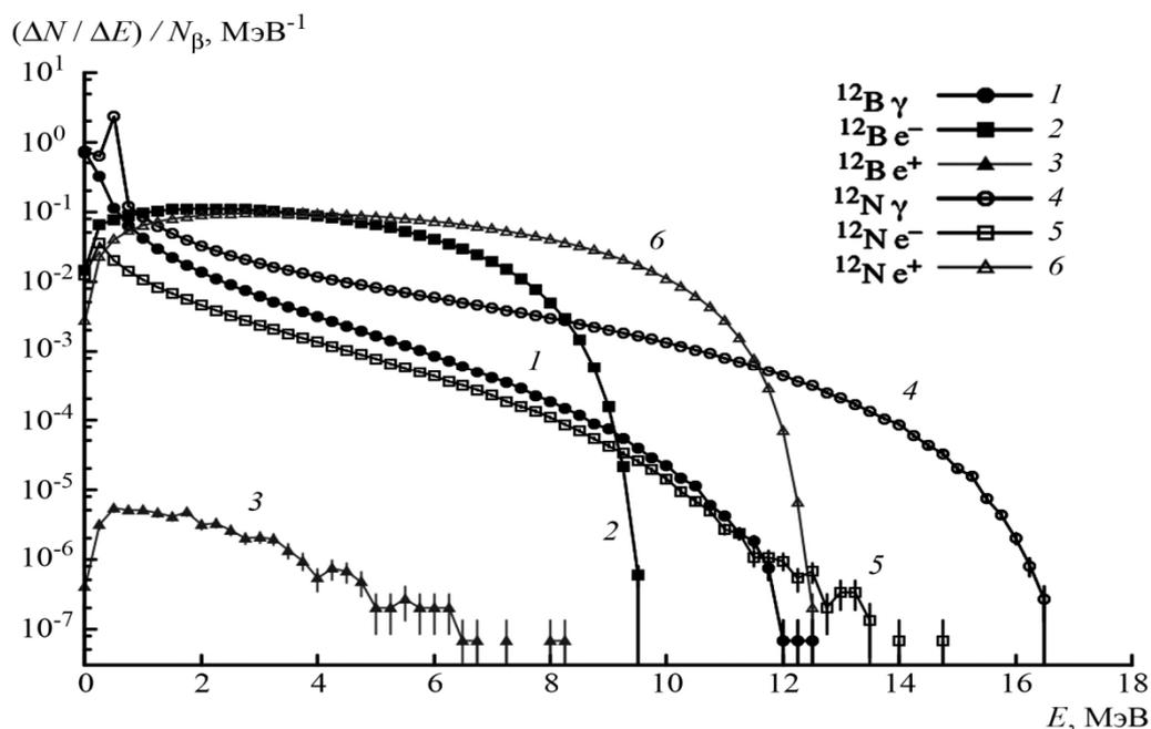
Fig. Calculated spectra of  $\gamma$ -quanta, electrons and positrons from sphere surface at  $\beta$ -decays of  $^{12}\text{B}$  and  $^{12}\text{N}$  from center of the sphere having  $\varnothing 20$  cm and containing equal quantities of H, C, N, O atoms at the total density  $0.25 \text{ g}\cdot\text{cm}^{-3}$ .
