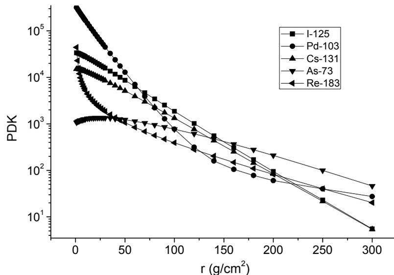
Fig. 1. Point dose kernel calculated for selected radionuclides.
