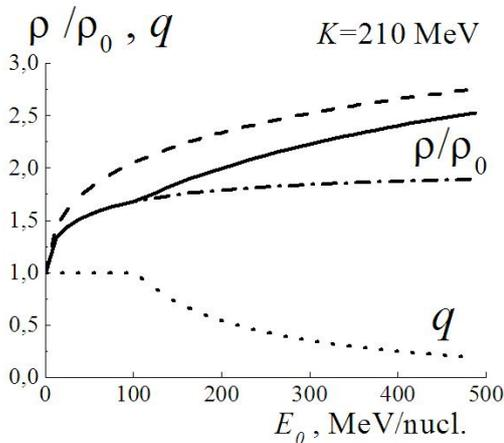
Fig.1. The energy dependence of the maximum compression ratio  $\rho/\rho_0$  of nuclear matter in the central collisions of Ar and Ca nuclei at the compression module  $K=210$  MeV (the solid line corresponds to the general case, the dashed line corresponds to the case of  $q=0$ , the dashed-dotted line corresponds to the case of  $q=1$ ), and the energy dependence of the relaxation factor  $q$  in the general case (the dotted line).
