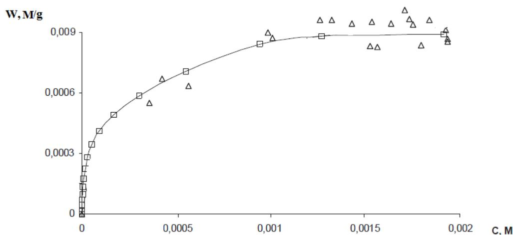
Fig. 1. Langmuir isotherm of dynamic adsorption of molybdate on alumina at 25°C.
